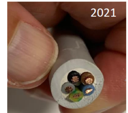
Picture 7: FG16OR16 5 X 1,5, cable manufactured according to CEI UNEL 35318 in 2021.
