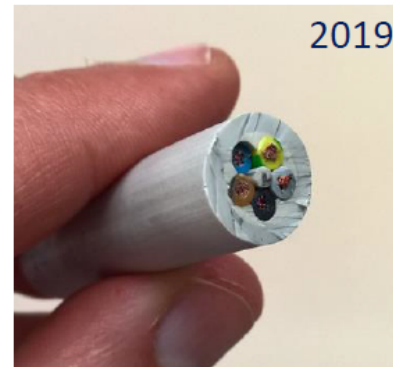
Picture 6: FG16OR16 5 X 1,5, cable manufactured according to CEI UNEL 35318 in 2019.
