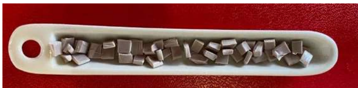
Figure 34: ceramic combustion boat according to EN 60754 series.
