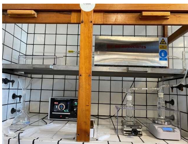
Figure 33: Tube furnace according to EN 60754 series.
