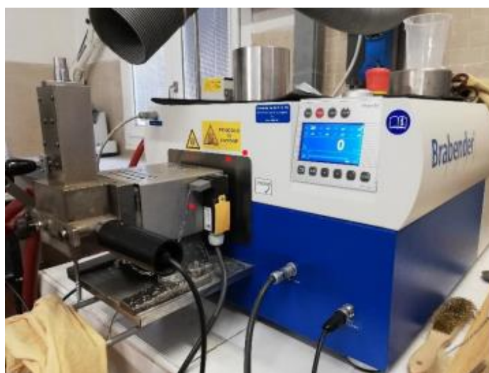
Figure 26: The plasticorder used (Brabender Plastograph EC + Mixer W50).
